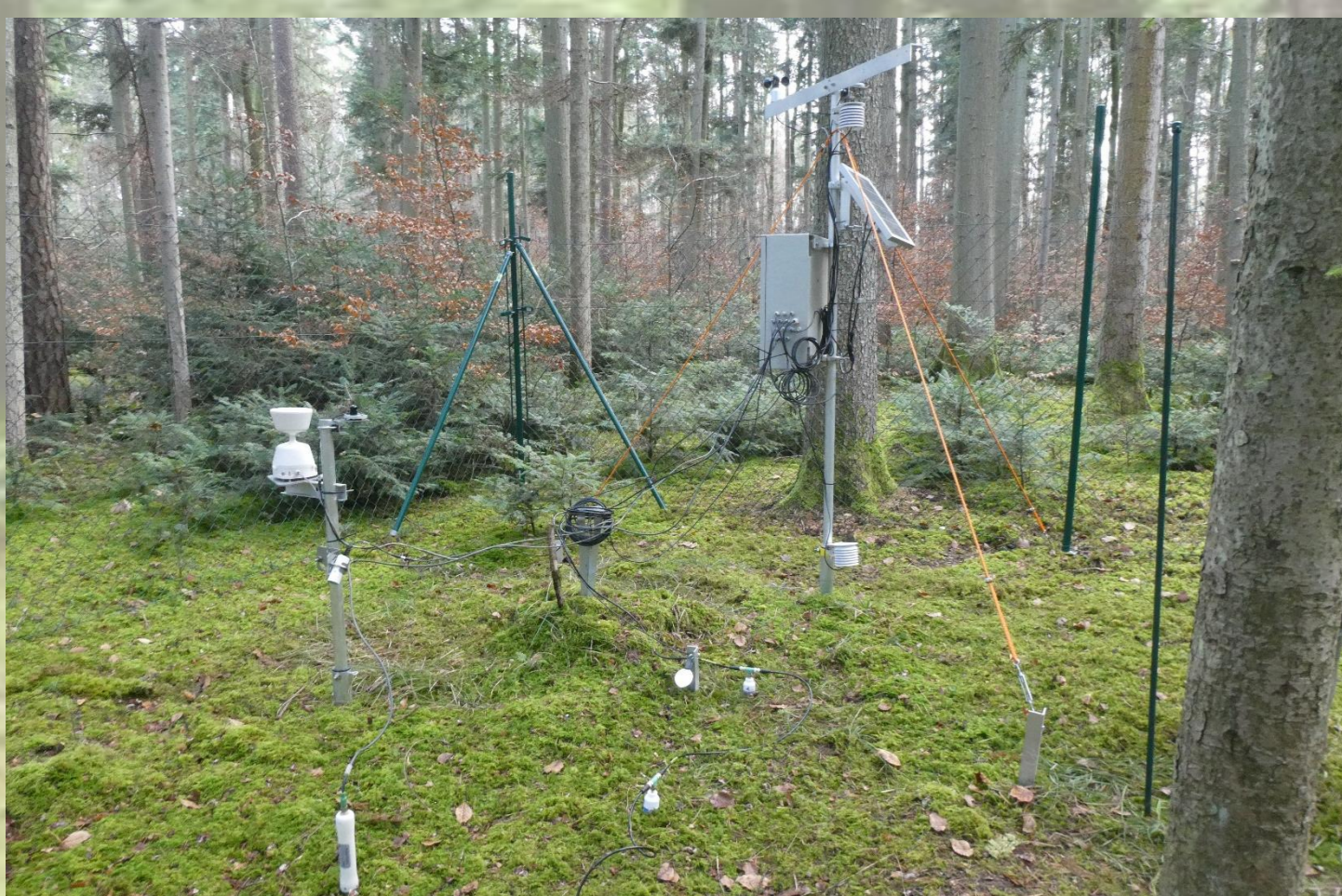
Continuous measurement of climatic, hydrological and soil parameters
