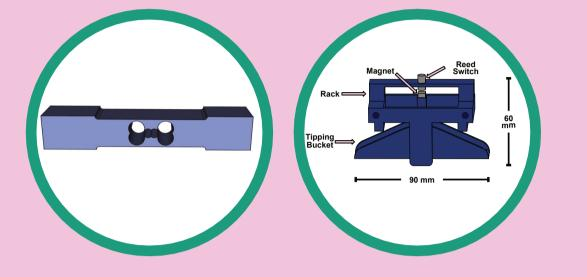
The load cells (LC) have a resolution of 6 g. After calibration, they show good accuracy. The temperature dependency, of the LC will be corrected using temperature sensors in and on the FFGL.
